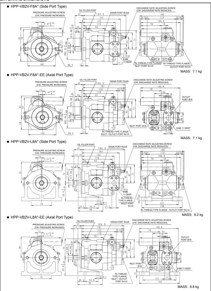
**NOTE:** Dimensions in parentheses are the dimensions of the welding type flange and those not in parentheses are the dimensions of the Rc thread type flange.
