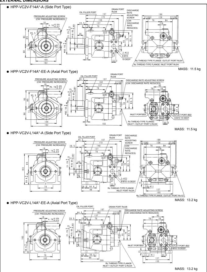
**NOTE:** Dimensions in parentheses are the dimensions of the welding type flange and those not in parentheses are the dimensions of the Rc thread type flange.
